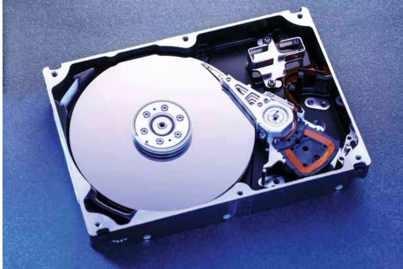
Figure 11.2 A 3.5-inch HDD with cover removed.
